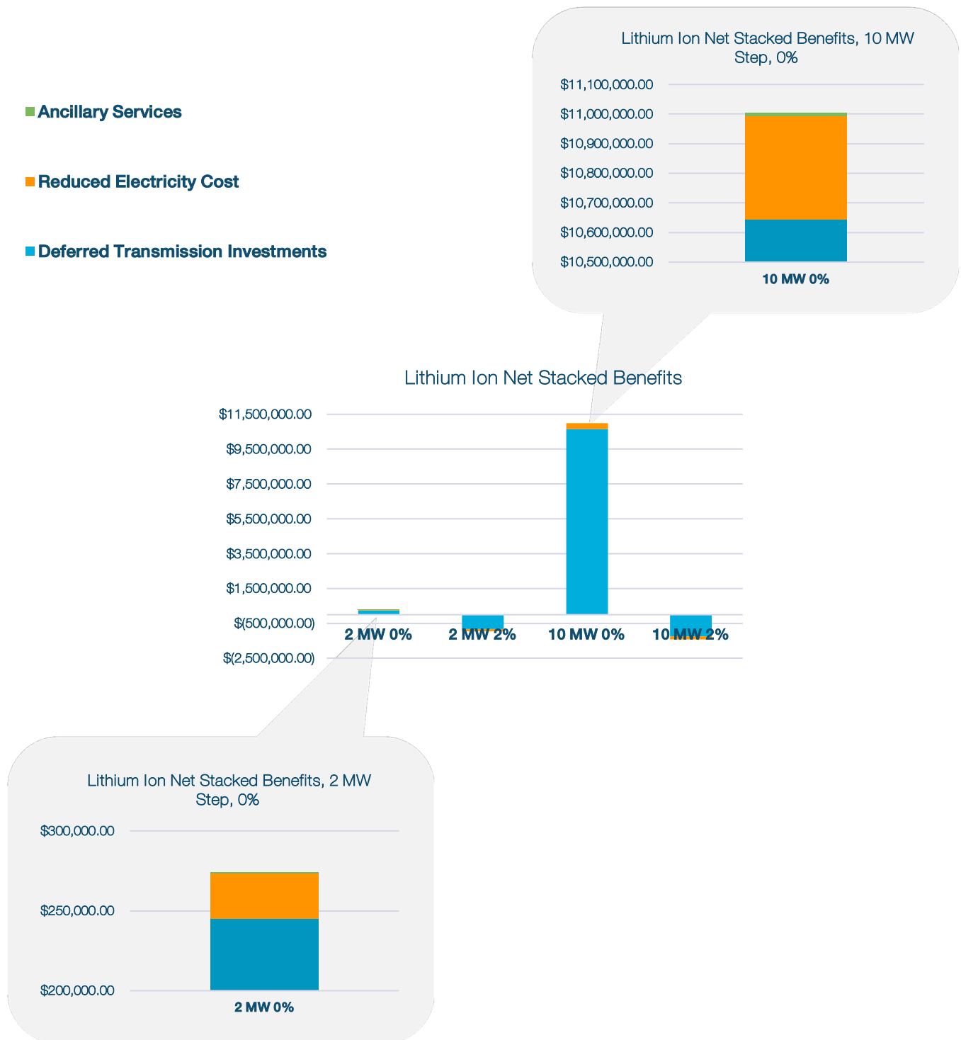
Figure 5: Computed Lithium Ion Net Stacked Benefits – Substantial Energy
